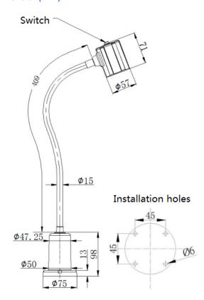
There is a magnet in the base of lamp, can adsorb on iron. In order to avoid to interference other electronic products, please keep the lamp base at least 100mm away from other electronic products.
